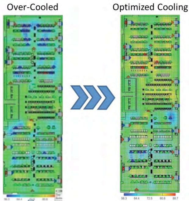
**Figure 3-11: Two Colo Rooms (Colo 9/10) Combined. Left Image: Over-Cooled, without the CRAH Fan Speed Control; Right Image: Temperatures Rise to the Desired 80.6°F (27°C) Temperature with the Speed Control, which Reduces CRAH Power.**
