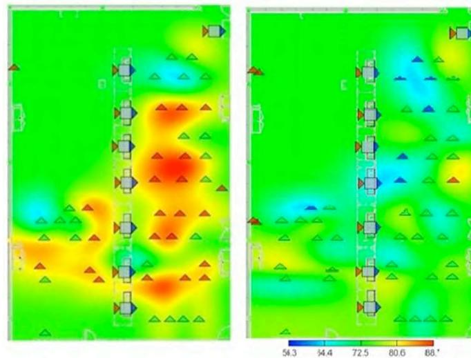
**Figure 3-8: Colo 2. Left Screen: Some Temperatures Above Limit; Right Screen: All Temperatures at or Below Set Point After Floor Tile Adjustments**
