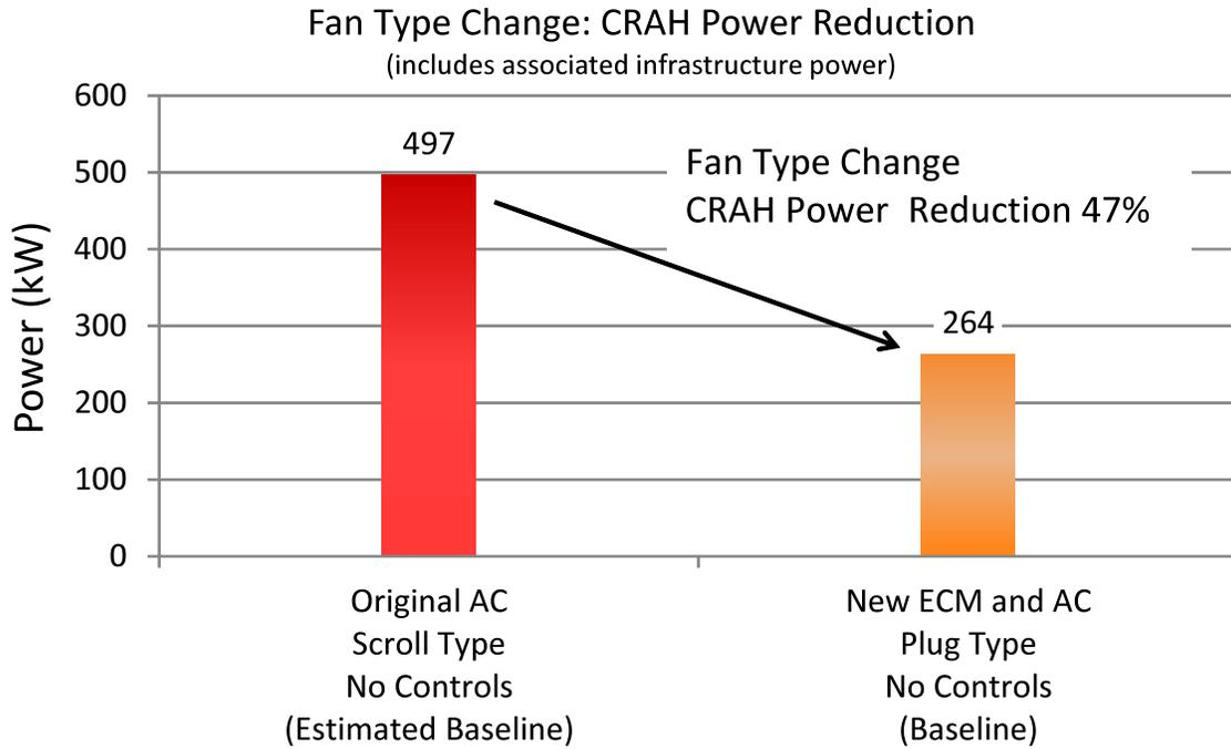
**Figure 3-1: CRAH Power Reduction (Including Associated Infrastructure Cooling Power) Due to Fan Upgrade from AC Scroll-Type to an Improved Efficiency AC and EC Motor Plug-Type**
