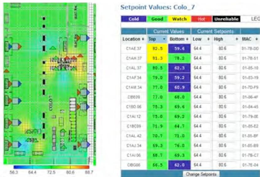
Figure 2-3: Example Data Center Floor Temperature Thermal Map and Set Point Status Screen
