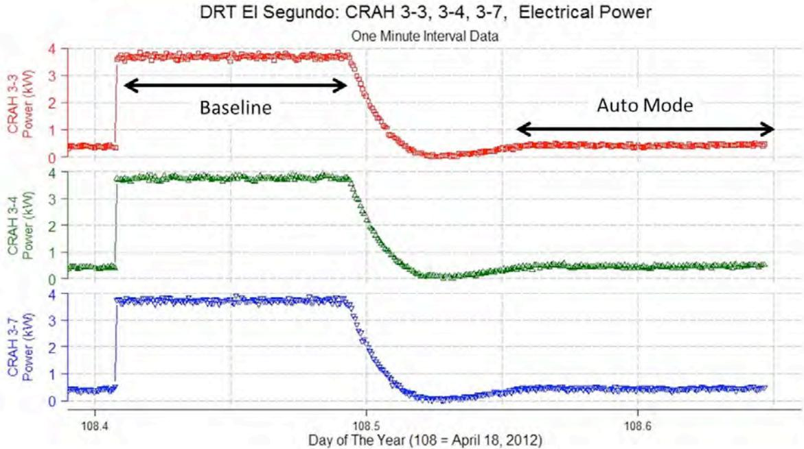
**Figure 3-6: Select CRAH Power Data from Colo 3, with High-Frequency Collected Data Shown During Baseline and Auto Mode Test Periods**
