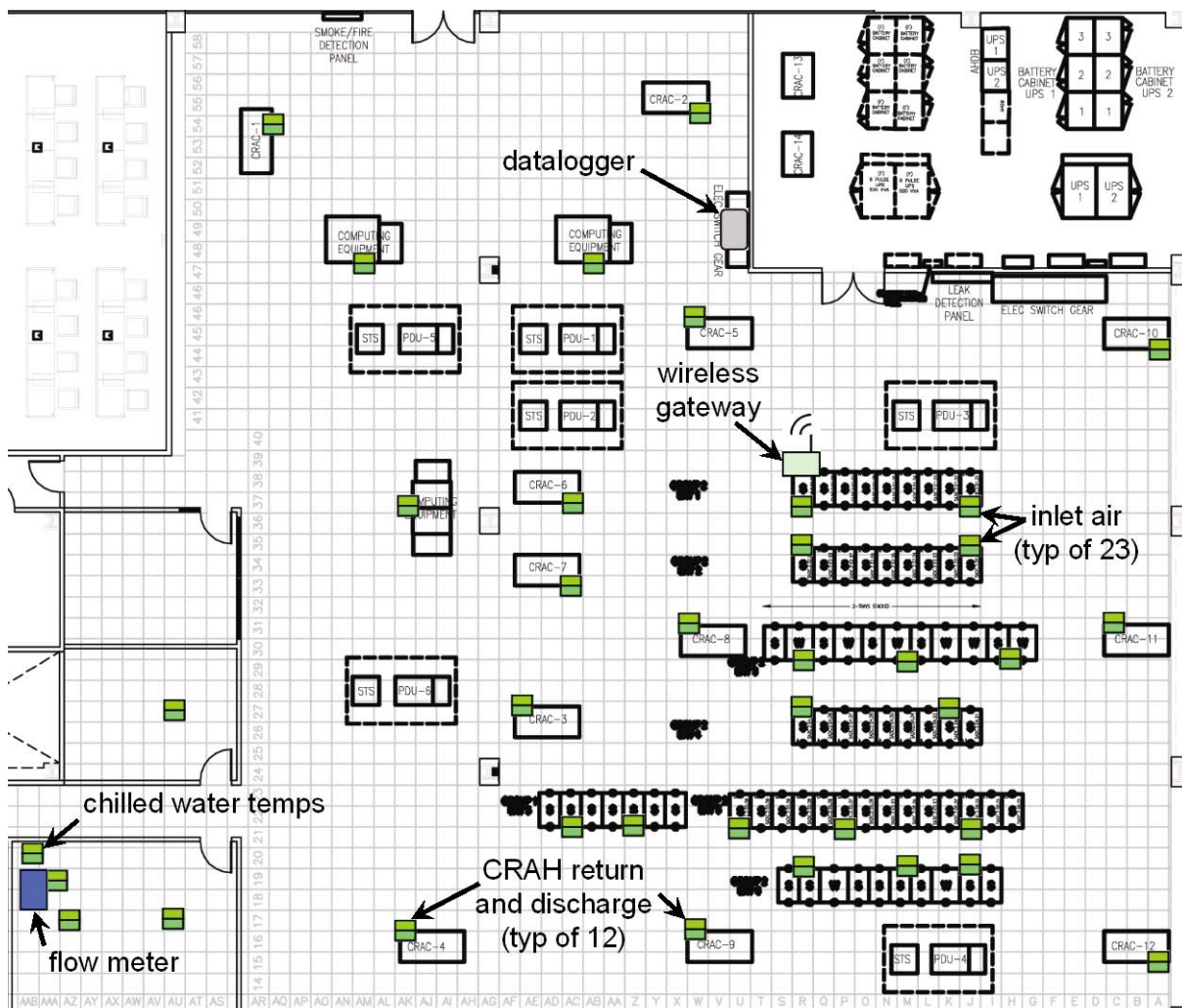
Figure 1: Floor plan with sensor locations.
