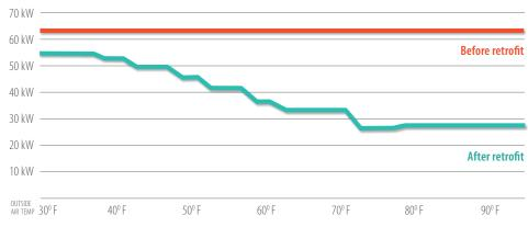
▲ The Vigilent Intelligent Energy Management System wireless HVAC retrofits at University Hall are contributing significant electricity demand savings. Compared to the previous constant air volume (CAV) system, which consumed an average of 63 kW when operating, the retrofit allows the system to reduce fan speeds and thus electricity consumption to match need throughout the building. These savings peak when the outside air temperature is 72-76° F.
