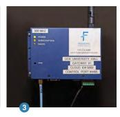
Two Vigilent wireless mesh gateways relay communications between the temperature sensors and the Vigilent Artificial Intelligence Engine.
